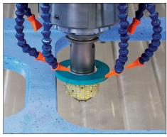
Contouring is used extensively when machining and polishing mouldings found on the edge of granite kitchen worktops. By supporting tool radius compensation, the diameter of the tool can be adjusted on the machine controller, thereby allowing for tool wear.
